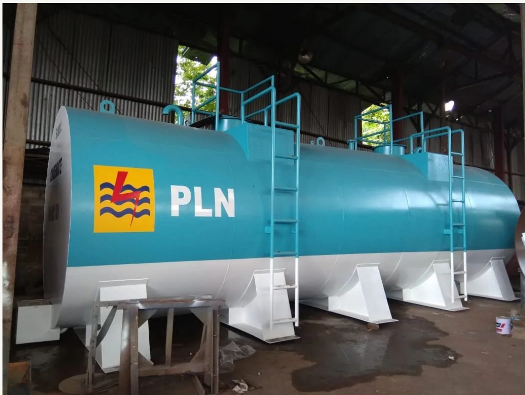
PLN 50 kL tank - company documentation.
